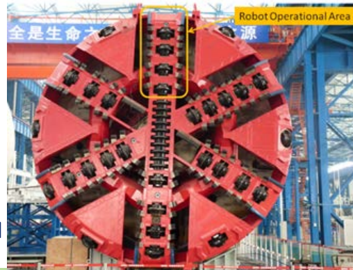
Semi-automatic device to change cutting discs in TBM
