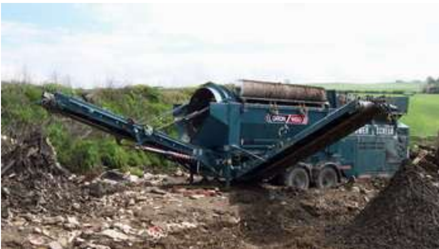
A Trommel screen used for recycling soil
