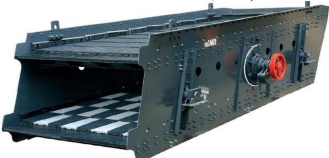
Screen with two decks
